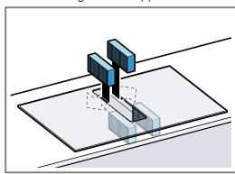
6. Insert the grease filter.
