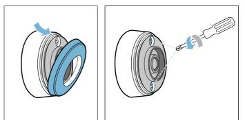
2. Open the closure of the temperature sensor. Remove the battery from the lower section of the housing and insert a new battery (pay attention to the correct orientation of the battery poles).
