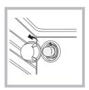
**3.** Reconnect the oven to the power supply. Note: Use 40 W/230 V type **G9**
