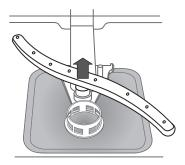
The lower spray arm may be removed by pulling it upwards.
