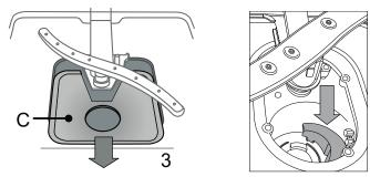
After cleaning the filters, re-place the filter assembly and fix it in position correctly; this is essential for maintaining the efficient operation of the dishwasher.
