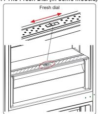
If the crisper is full, the fresh dial located in front of the crisper should be opened. This allows the air in the crisper and the humidity rate to be controlled, to increase the life of food within.
