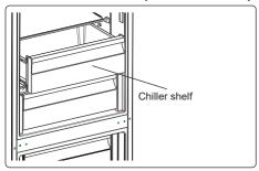
Keeping food in the Chiller compartment, instead of the freezer or refrigerator compartments, allows food to retain freshness and flavour for longer, while preserving its fresh appearance. When the Chiller tray becomes dirty, remove it and wash with water.
