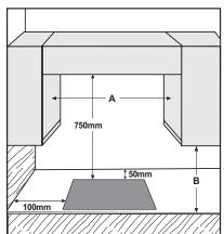
NOTE: if distance "A" between the kitchen cabinets is between 600 mm and 730 mm, height "B" must be at least 530 mm. If distance "A" between the kitchen cabinets is greater than the width of the hob, height "B" must be at least 400 mm. If a hood is installed above the hob, refer to the assembly instructions for the hood to see the necessary distance.
