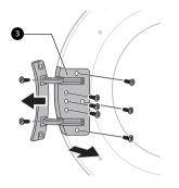
3 Remove the 3 screws from the door latch assembly which is fixed between the door and the hinge assembly, and then remove the screw which is fixed on the door hook.
