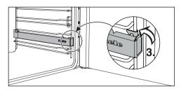
■ Then secure the FlexiClip runner to the bottom of the two rails as illustrated (3).
