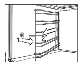
■ Pull the runners out of holder (1) at the front of the oven and then pull them out of the oven (2) together with the catalytic side liners (if fitted).
