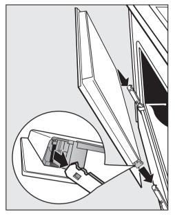
Hold the door securely at both sides and carefully fit it back onto the hinge retainers. Make sure it goes on straight. ■ Open the door fully.
