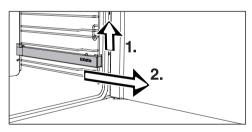
■ Remove the FlexiClip runner by raising it at the front (1.) then pulling it forwards along the rail and out (2).
