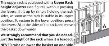
just the height of the rack when it is loaded. NEVER raise or lower the basket on one side only.
