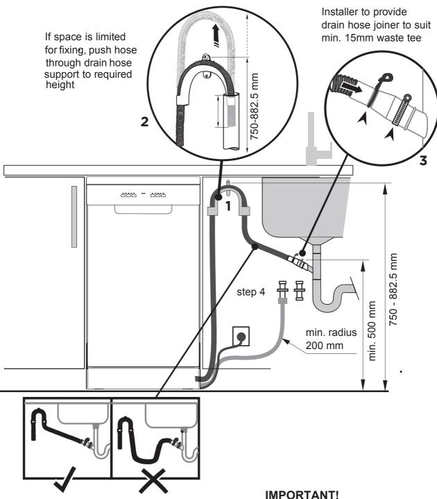
Ensure drain hose is routed straight to joiner. Remove excess drain hose material if necessary. Do not shorten the inlet hose.
