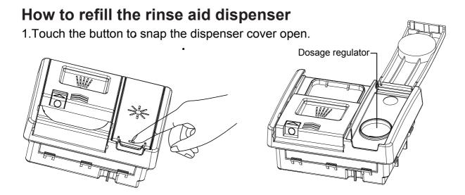
2. Pour rinse aid into the circular opening, making sure not to fill beyond the MAX marking.
