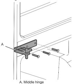
Lift freezer door from bottom hinge pin.
