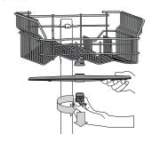
To remove the upper spray arm, turn the plastic locking ring in an anti-clockwise direction. The upper spray arm should be replaced so that the side with the greater number of holes is facing upwards.
