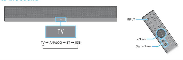
Press INPUT repeatedly until the device you want appears in the top panel display. Then, press 4+/- repeatedly to adjust the volume of the system and press SW 4+/- repeatedly to adjust the volume of the subwoofer.
