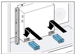
14. Plug the cables into the fan box.
