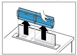
**3.** Remove the grease filters. To avoid causing damage, do not bend the grease filters.
