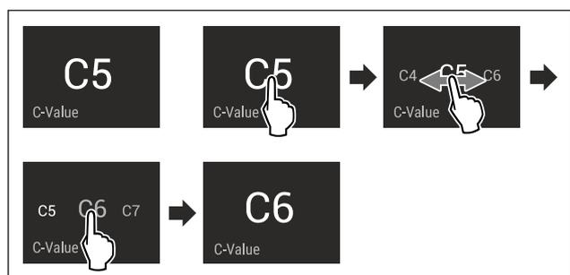
Fig. 21 Example illustration: Switch from C5 to C6.
