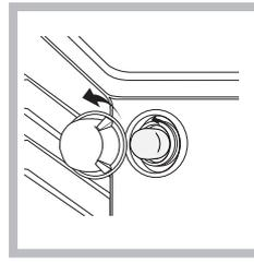
1. After disconnecting the oven from the electricity mains, remove the glass lid covering the lamp socket (see figure).
