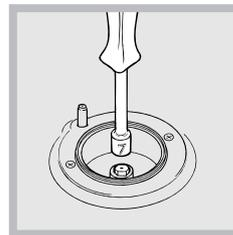
Replacing the nozzles for the hob burners:
