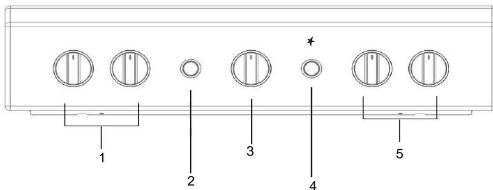
1. Control Knobs for Gas Burners on Hob
