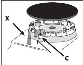
Several models are equipped with an ignition device which is built into the knob; in this case the electronic ignition device\* is present (see figure) but the ignition button is not. Simply press the BURNER knob and turn it in an anticlockwise direction so that it is pointing to the maximum flame setting, until the burner is lit. The burner may be extinguished when the knob is released. If this occurs, repeat the operation, holding the knob down for a longer period of time.
