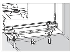
■ Screw in adjustable feet ② completely.
