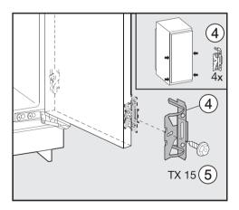
Screw fixing bracket 4 using hex screw 5 to the pre-drilled holes in the appliance door.
