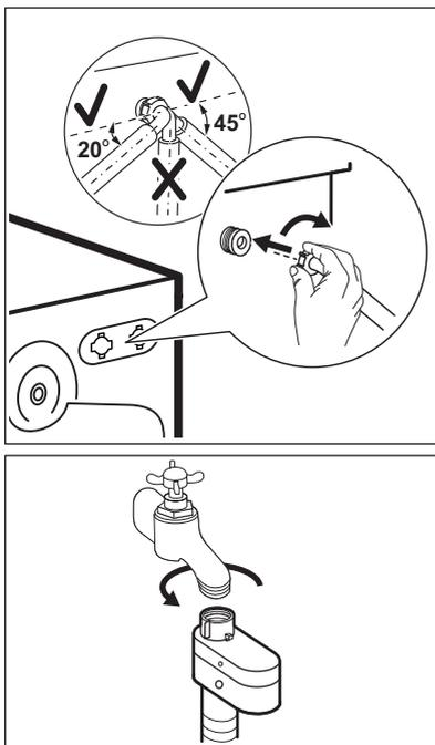
3. Connect the hose to the back of the appliance. Do not turn the inlet hose downwards, but turn it left or right depending on the position of your water tap.
