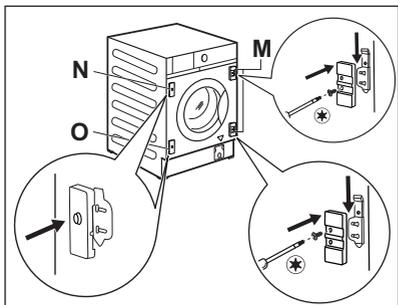
**i** Make sure that the plate with magnet is on the upper position.
