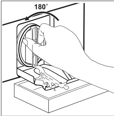
3. Turn the filter 180 degrees in anti-clockwise direction to open it, without removing. Let the water flow out.
