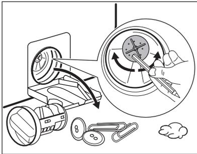
7. If it is necessary, remove fluff and objects from the filter recess. Make sure that the impeller of the pump can rotate. If it does not rotate, contact the Authorised Service Centre.
