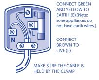
If the colours of the wires in the mains lead of this appliance do not correspond with the coloured markings identifying the terminals in your plug, proceed as follows:
