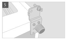
Tilt the fridge back, no more than 45°, to access the bottom hinge and feet. Remove the feet and the bolts securing the right hand hinge plate and the left hand fixing plate.
