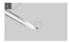
Remove the four blanking plates from the top of the fridge with a flat bladed screwdriver. Remove the screws underneath with a Phillips screwdriver.
