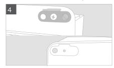
Remove the hinge insert plate from the bottom of fridge door. Replace the plate on the opposite side.
