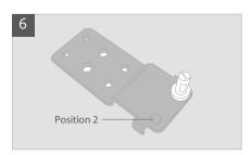
Remove the hinge pin from position 1 and replace it in position 2. Place the hinge on the opposite side of the cabinet, secure it with the three bolts, and screw in the foot into position.
