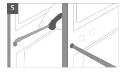
Remove the blanking plates and screw cover. Remove screw and replace screw on the opposite side.
