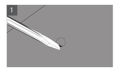
Remove the four blanking plates from the top of the fridge freezer with a flat blladed screwdriver. Remove the screws underneath with a Phillips screwdriver.
