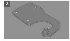
Use the 8mm socket or spanner to remove the three bolts above the door hinge. Lift off the bracket. Remove the fridge door.
