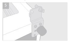
Tilt the fridge back, no more than  $45^\circ$ , to access the bottom hinge and feet. Remove the feet and the bolts securing the right hand hinge plate and the left hand fixing plate.
