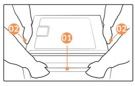
Be sure to hold the appliance with 2 side handles and door handle when unpacking the product.
