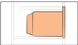
2. Slide the oven completely into the recess.
