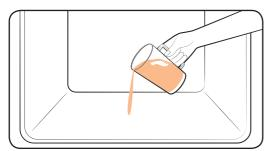
**3.** Pour 100 ml of water onto the bottom of the oven and close the oven door, and then tap **OK**. It takes 15 minutes to complete the cycle.
