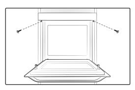
**3.** Fasten the oven using the two screws (4 x 25 mm) provoded.
