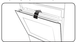
The door starts to be closed softly at about 15 degrees and completely closed within approx. 5 seconds.
