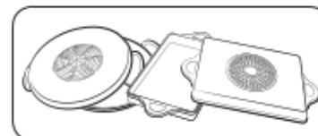
When using large cookware with a smaller ferromagnetic element, only the ferromagnetic element heats up. Consequently, heat might not be uniformly distributed.
