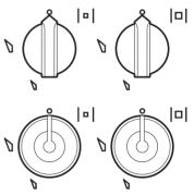
Double-crown burners comprise an auxiliary and a rapid burner. It is controlled by two different knobs which permit to use both burners at the same time or to select one or the other as required.
