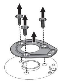
5. The two rear screws need to be removed only on 70 cm models.
