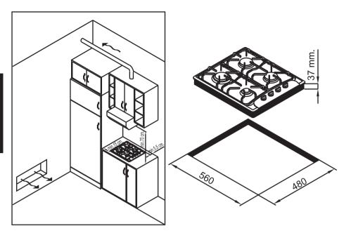
The body of the hob is fitted with 4 location holes to take the fixing brackets that secure the hob in the unit. Place 4 fixing brackets in such a way that the hob is placed perfectly in the support unit.
