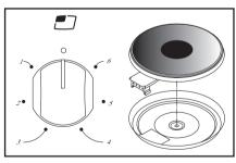
Turn the knob to the position for the required temperature of the hot plate. The indicator light of the hot plate will come on and the hot plate will start to heat.
