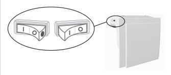
When the ionizer is switched on, a red dot will be visible on the switch.
