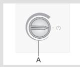
To switch on: rotate the A dial clockwise.
