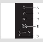
If the temperature inside the appliance is too high, acoustic alarm will be activated (**intermittent tone**) and the **B** key will flash.
