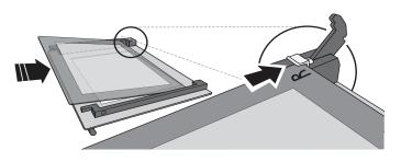
**4.** Refit the upper edge: A click will indicate correct positioning. Make sure the seal is secure before refitting the door.
