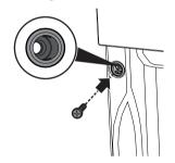
4. Cover the bushings with the previously removed covers.
