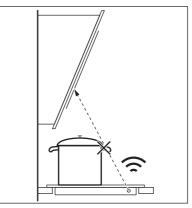
i Other remotely controlled appliances may block the signal. Do not use any remotely controlled appliances at the time when you use the function on the hob.
