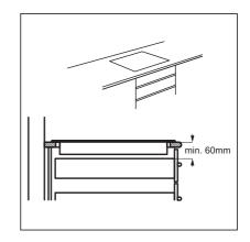
i If the appliance is installed above a drawer, the hob ventilation can warm up the items stored in the drawer during the cooking process. You can instal a separation panel but it is not mandatory.
