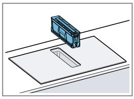
3. Remove the four odour filters or acoustics filters, and dispose of them properly.
