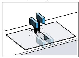
6. Insert the grease filter.
