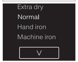
■ Touch the ∨ sensor to select the drying level required. Any drying level can be selected for the *Cottons* programme. A more limited range is available when using the other programmes.
