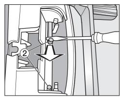
■ Use the screwdriver to guide first one then the other rod ② to the middle until each can be removed.
