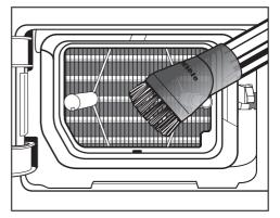
Carefully vacuum up any visible fluff or soiling.
