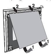
Clean the external glass panel and the panels previously removed. Use absorbent kitchen roll. In case of stubborn dirt, wash with a damp sponge and neutral detergent.
