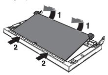
4. Clean the external glass panel and the panels previously removed. Use absorbent kitchen roll. In case of stubborn dirt, wash with a damp sponge and neutral detergent.
