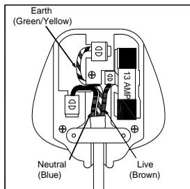
This appliance is equipped with a plug fitted with a 13 amp fuse. Should the fuse fail, then it must be replaced with an ASTA approved fuse (conforming to BS1362) of the same rating. If you need to replace the plug or if the plug is of the incorrect type for your socket, remove it and replace it with an appropriate type. Dispose of the old plug safely.
