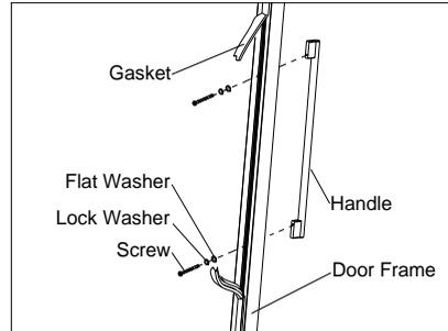
1. Remove the door gasket on the side you wish to install the handle - you can see two designated holes for handle installation.
