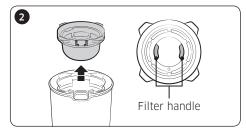
Pull the washable micro filter out by holding the filter handles inside the washable micro filter
