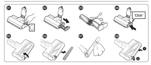
If the foreign matter is not removed, use scissors to remove it.
