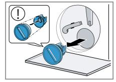
2. Clean the interior, the thread on the pump cap and the pump housina.
