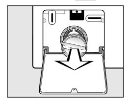
■ Remove the drain filter completely.
