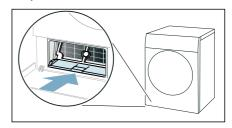
**10.** Slide the heat exchanger cover in by its grip.
