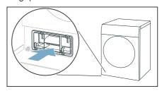
**Note:** You can only slide the heat exchanger cover in if the insert is in the appliance.
