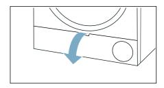
3. Unlock the levers on the heat exchanger cover.
