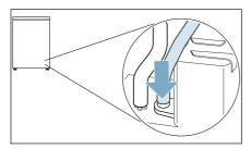
**6.** Push the drain hose into the appliance's hose guide.
