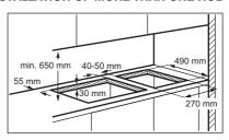
If several 30 cm hobs are to be installed side by side into the same cut out, an assembly kit including a support side bracket and supplementary seals is available at our Authorised Service Centres. The relevant installation instructions are supplied within the kit package.
