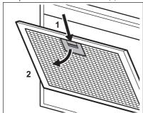
Slightly tilt the front of the filter downwards (2), then pull.
