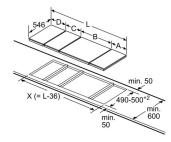
When installing several elements side by side, several assembly kits are also required (Z9914X0).
