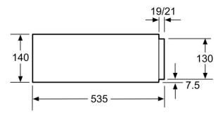
Compact ovens with an appliance height of 455 mm can be installed above a warming drawer.
