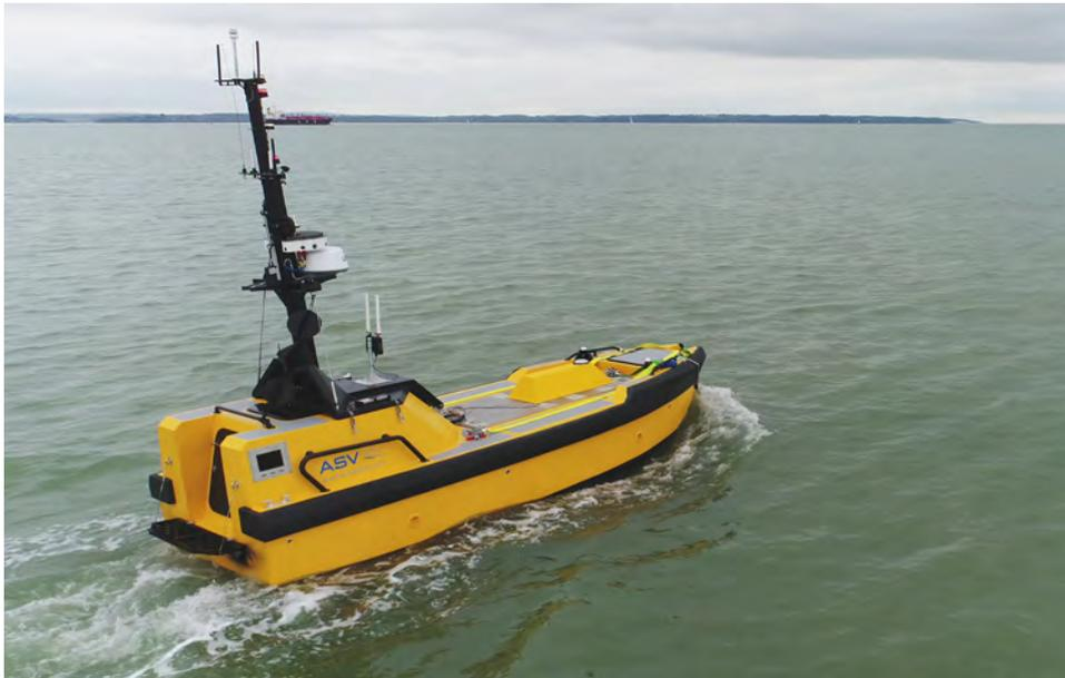
Figure 2: ASV Global's C-Worker 7 autonomous surface vessel.
