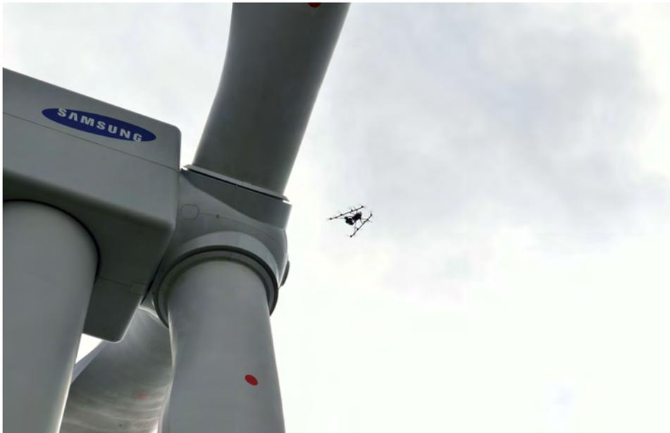
*Figure 1: UAV blade inspection*
