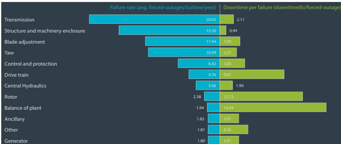
Figure 2: Analysing performance by looking at failure rates and downtime per failure.
