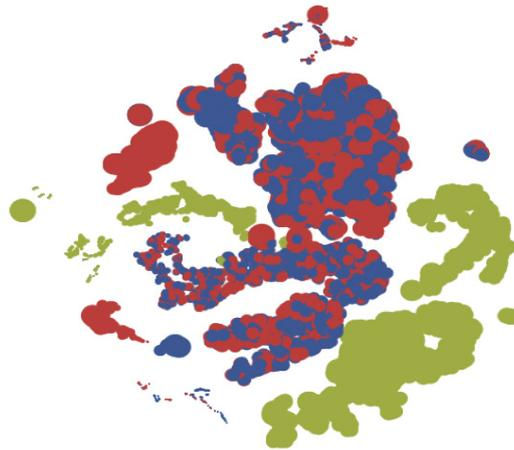
*Figure 3: Result of dimension reduction of SCADA signals by machine learning algorithms, showing two turbines performing similarly (red and blue) and one that is different (green).*
