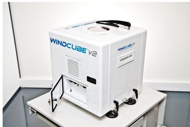
The big advantage of LiDAR systems relies in their quick and easy deployment. This can be especially interesting at isolated and complex sites where high masts installation (>80 m height) can be very challenging (and expensive). WINDCUBE v2 LiDAR is the optimal choice for complex terrains as its Flow Complexity Recognition (FCR) feature ensure the measured data is IEC-class 1 accurate even in the most complex terrains.
