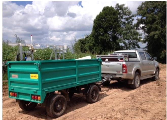
The WINDCUBEv2 LiDAR was installed 8 m away from each met mast and the LiDAR moved around the site as per the schedule. In order to minimize the monitoring location shifting times (especially when the shifting frequency is very high), MeteoPole strongly recommended placing the LiDAR device on a moving vehicle. This was done by fixing the LiDAR on a trailer as it can be seen on the picture.
