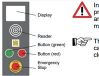
In the event of danger, press EMERGENCY STOP and switch off the coloured main switch!
