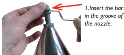
1. Insert the bar in the groove of the nozzle.
