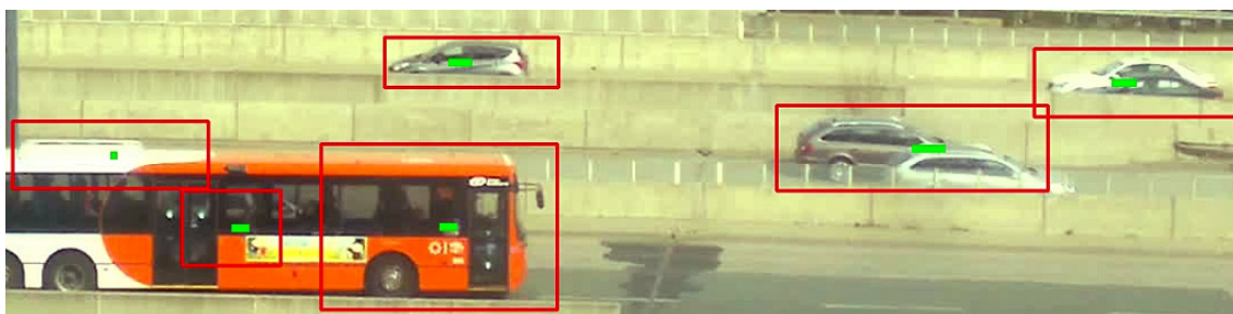
Figure 2: A problematic video frame with a bus counted as three separate cars, and a few cars are merged together. The bus problem wouldn't occur with a better background separation algorithm.
