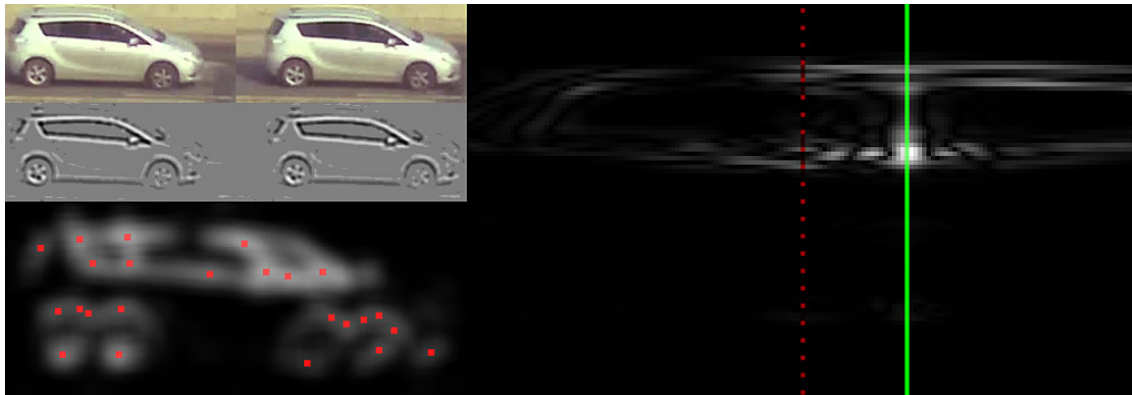
Figure 3: A single car detection and velocity measurement example. The difference between frames is visualized in lower left corner, and red points indicate local difference maxima. The image on the right visualizes the cross-correlation for different image rows and offsets, mid-point is indicated in red and the maximum correlation is indicated by the green line.
